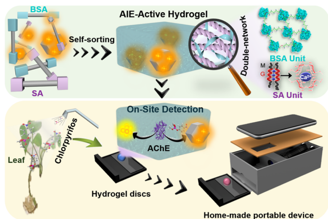
Scheme 1. Schematic Illustrations of AIE-Active Hydrogel Discs for Pesticide Detection
