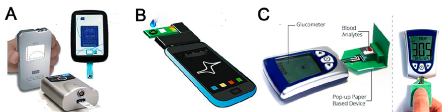
Figure 2. Portable electrochemical sensors: (A) commercially available pocket-sized potentiostats. Adapted with permission from ref 87. Copyright 2017, Wiley-VCH. (B) Smartphone-based potentiostats. Adapted with permission from ref 87. Copyright 2017, Wiley-VCH. (C) Routine blood glucose meter. Reproduced with permission from ref 90. Copyright 2016, American Chemical Society.
