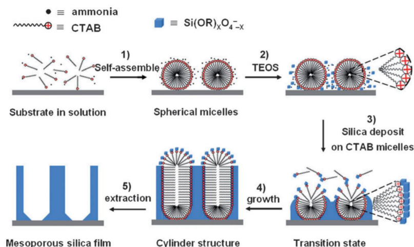
Figure 13. Schematic illustration of the Stober solution growth mechanism (SSG) used to create silica nanochannel membranes: (A) substrate in solution self-assembling into spherical micelles, (B) reaction of TEOS with the template of micellar rods, (C) silica deposited on CTAB micelles and spherical structure transitioning into a cylindrical structure, (D) growth of the cylindrical structure, and (E) extraction of the CTAB to create silica nanochannels. Reproduced with permission from ref 147. Copyright 2012 WILEY-VCH Verlag GmbH & Co. KGaA, Weinheim
