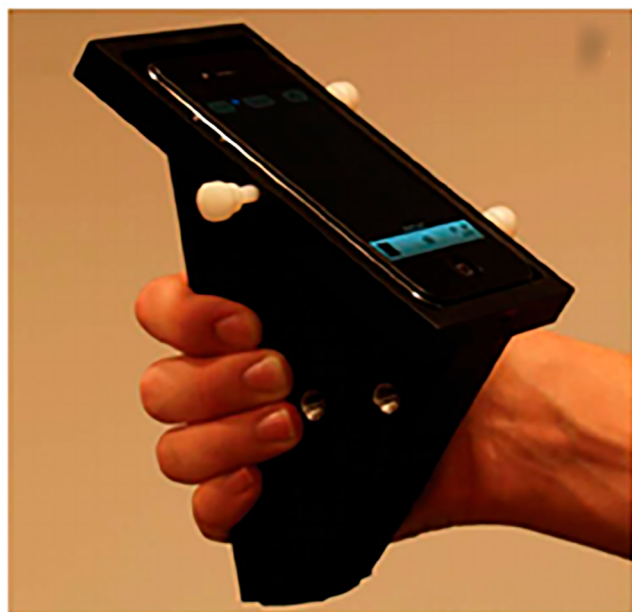
Figure 7. Cradle accessory for a smartphone used to control photographic conditions for optical sensing. Reprinted in part with permission from ref 69. Copyright 2013 Royal Society of Chemistry.
