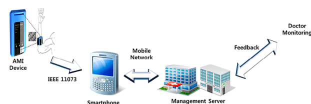
Figure 3. Wireless data transmission from a mobile biosensor for acute myocardial infarction (AMI) to a smartphone using a standard protocol for health data (IEEE11073). From the smartphone, data is transmitted to a server at a healthcare facility where it can be securely accessed by a doctor for review. Reprinted in part with permission from ref 35. Copyright 2015 Wiley Online Library.
