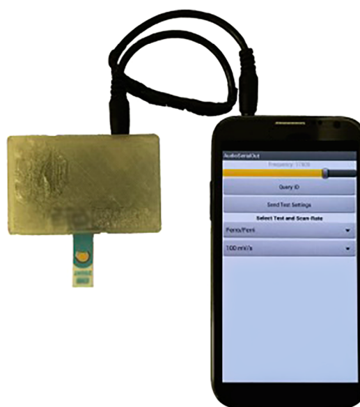
Figure 6. Biosensor dongle that connects directly to a smartphone and harvests power via the headphone jack, eliminating the need for a separate battery. Reprinted in part with permission from ref 52. Copyright 2016 Elsevier.
