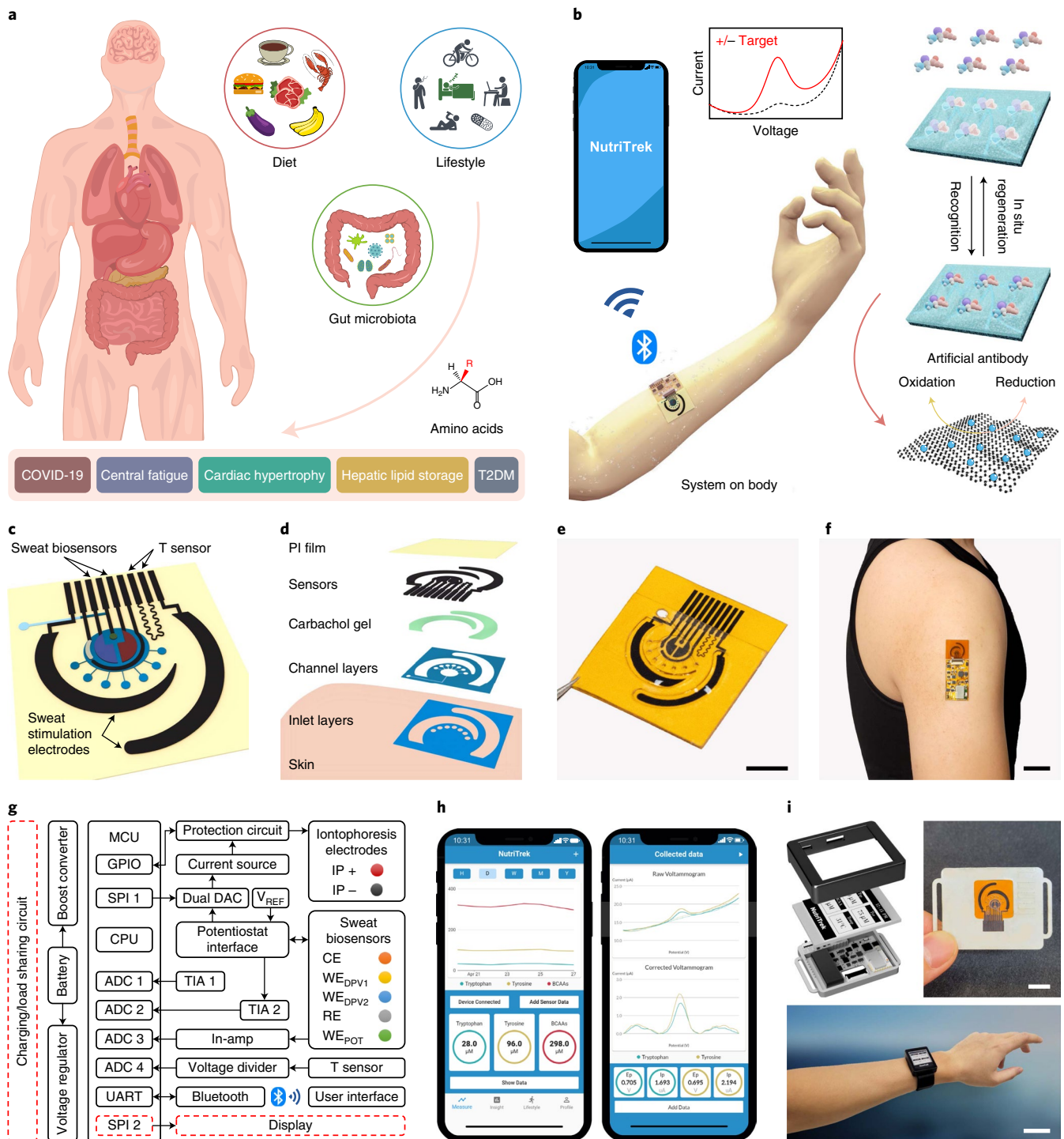
Fig. 1 | Schematics and images of the wearable biosensor 'NutriTrek'. a , Circulating nutrients such as AAs are associated with various physiological and metabolic conditions. b , Schematic of the wearable 'NutriTrek' that enables metabolic monitoring through a synergistic fusion of LEG, RARs and artificial antibodies. c,d , Schematic ( c ) and layer assembly ( d ) of the microfluidic 'NutriTrek' patch for sweat induction, sampling and biosensing. T, temperature. e,f , Images of a flexible sensor patch ( e ) and a skin-interfaced wearable system ( f ). Scale bars, 5 mm ( e ) and 2 cm ( f ). g , Block diagram of electronic system of 'NutriTrek'. The modules outlined in red dashes are included in the smartwatch version. CPU, central processing unit; POT, potentiometry; In-Amp, instrumentation amplifier; MCU, microcontroller; TIA, trans-impedance amplifier; IP, iontophoresis; CE, counter-electrode; RE, reference electrode; WE, working electrode. h , Custom mobile application for real-time metabolic and nutritional tracking. i , 'NutriTrek' smartwatch with a disposable sensor patch and an electrophoretic display. Scale bars, 1 cm (top) and 5 cm (bottom).
