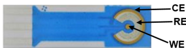
Figure 1. Gold sensors (BVT technologies, AC1W1R1) showing counter electrode (silver), reference electrode (carbon) and working electrode (gold).
