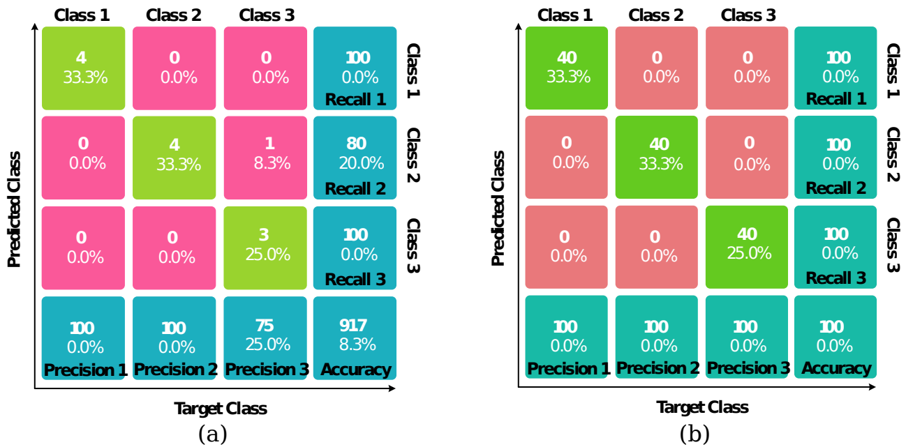
Figure 16. Confusion matrix of the neural network classifier for tissue type detection using sensor output parameters. The matrix compares predicted classes (vertical axis) against true labels (horizontal axis). Class 1 = Healthy, Class 2 = HPV-infected, Class 3 = Cancerous. (a) Original dataset, and (b) augmented dataset.
