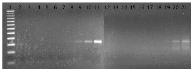
Fig. 3 Effect of thin film biosensor on HDA amplification rate. effect of thin film biosensor on HDA amplification rate. HDA reactions were performed on 1000 copies of MRSA genomic DNA on the thin film biosensor surface. Aliquots (10 \mu L) were removed and subjected to electrophoresis on 2% agarose gel. Lanes 1–11: amplification reactions on thin film biosensor, lanes 12–21: amplification reactions in tubes. Lane 1: 25 bp ladder; lane 2, blank; lanes 3 and 13, negative control at 20 min.; lanes 4 and 14, negative control at 35 min.; lanes 5 and 15, 20 min. reaction; lanes 6 and 16, 22.5 min. reaction; lanes 7 and 17, 25 min. reaction; lanes 8 and 18, 27.5 min. reaction; lanes 9 and 19, 30 min. reaction; lanes 10 and 20, 32.5 min. reaction; lanes 11 and 21, 35 min. reaction.
