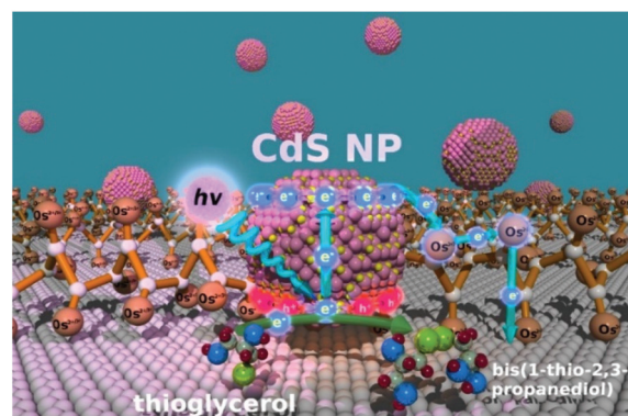
Scheme 1 Detection of CdS QDs on the screen-printed carbon electrode modified with an osmium polymer under UV irradiation.
