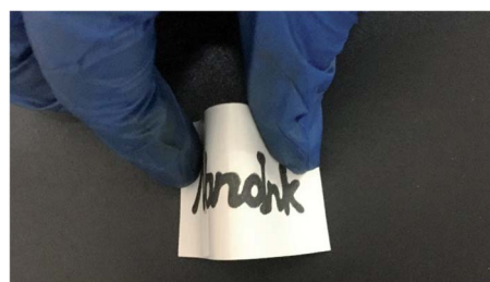
Fig. 2 Display of the flexibility of the Ag@Au core-shell/GQD nano-ink drawn on the surface of the photographic paper.
