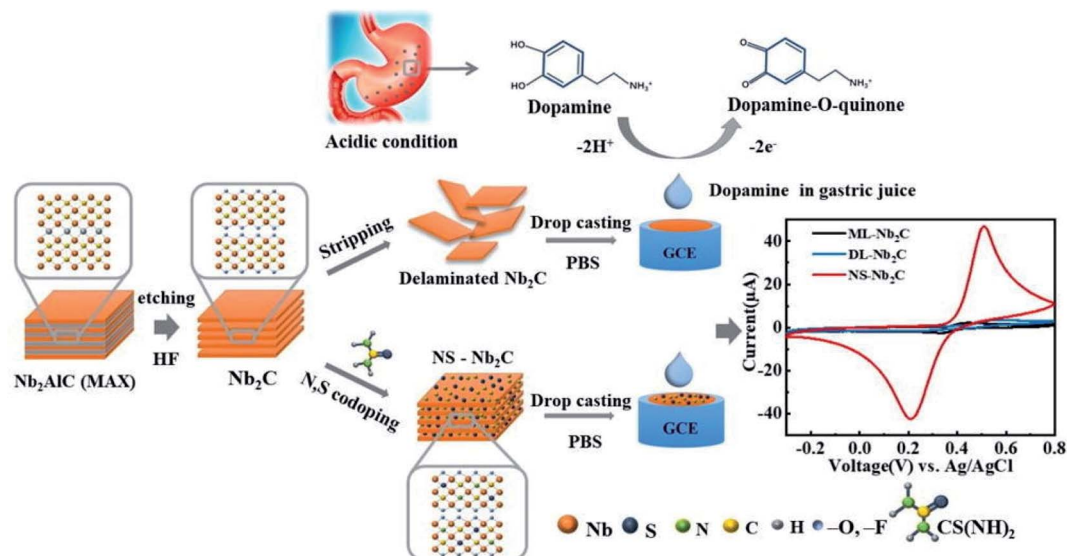
Fig. 10 Schematic synthesis of N,S co-doped Nb 2 C MXene and assembly for DA sensing in acidic condition. CV curves on the right side shows that the redox current peaks in case of N,S co-doped Nb 2 C sheets are greatly enhanced as compared to multilayered (ML) or delaminated (DL) Nb 2 C MXene. Due to high electron transfer rate and surface area expansion for molecular interaction imparted by N,S doping. Reproduced from ref. 178 after permission, copyright© 2021 Elsevier.
