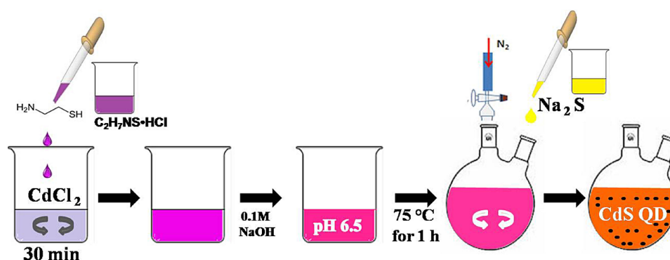
Fig. 2 Schematic representation of CdS quantum dot synthesis
