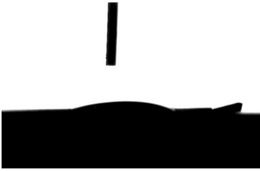
Figure 7. The contact angle of Pt/PPy-DBS-ChOx.
