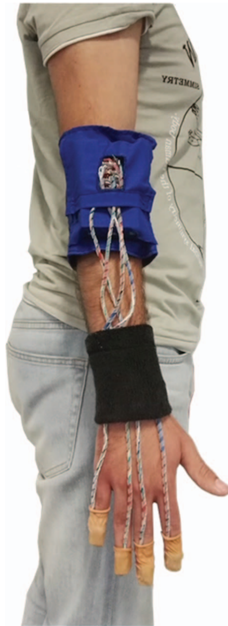
Figure 1. Device positioning: accelerometers were placed on hand's fingers.
