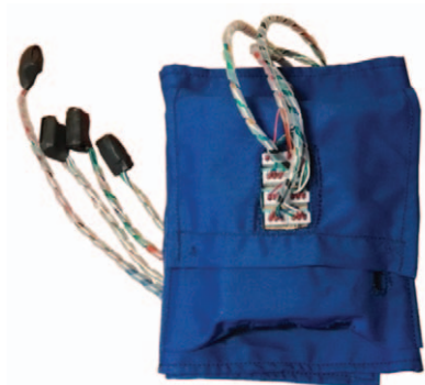
Figure 3. Three-dimensional printed enclosure with 4-accelerometer array.
