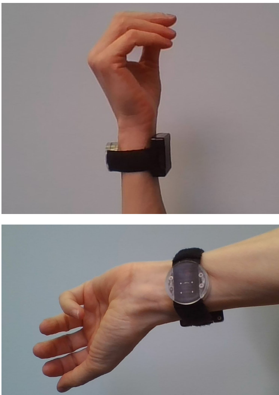
Figure 1. Pictures of WrisTAS™ being worn on wrist: clear disc contains the sensors; black box contains electronics and battery.
