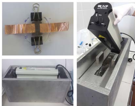
Figure 1. Experimental setup for irradiation of the nanomaterial-based sensors by UV light. The closed irradiation chamber with the UV lamp integrated in the lid is shown in the picture on the right. The assembly of the sensor surface between the glass bottom substrate and the PDMS top substrate is in the upper left picture.
