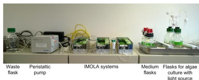
Figure 4. Measurement setup and flasks for algae culture.
