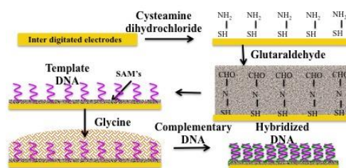
Figure 2: Schematic representation of immobilization technique.
