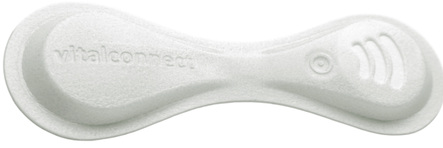
Fig. 1: A fully disposable VitalPatch sensor worn on chest allows seamless 24 hour patient monitoring.
