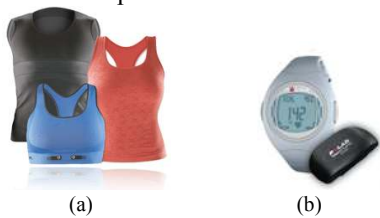
Fig. 1. Numetrex smart garments with embedded ECG electrodes (a), and a compatible Polar transmitter and wristwatch (b).
