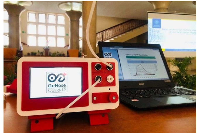
Fig. 9. Photograph of GeNose device. Reprinted from [117] with permission from Gadjah Mada university press.
