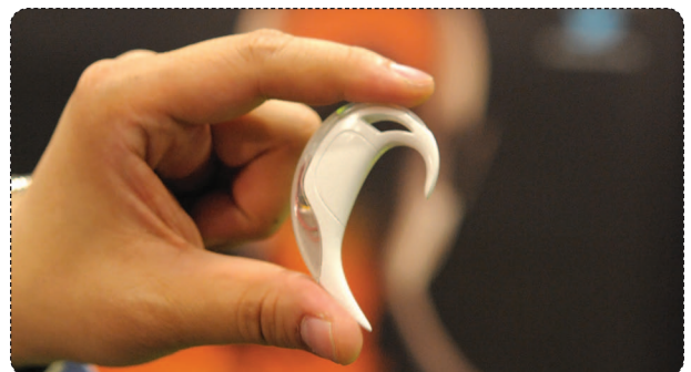
FIGURE 6 Yang and his group designed the award-winning e-AR sensor. Inspired by the function of the human inner ear, this small device fits discreetly behind the ear and captures similar information, i.e., the balance of the wearer. With advanced signal processing, further information about the gait, posture, skeletal/joint shock-wave transmission, and activity of the individual can be deduced. (Photo courtesy of Sensixa Ltd.)
