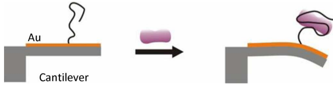
Fig. 9. Basis of cantilever biosensors. Microfabricated silicon cantilevers are coated in a thin gold layer to which aptamers are attached. Target binding causes a deflection in the cantilever, which can be detected optically.
