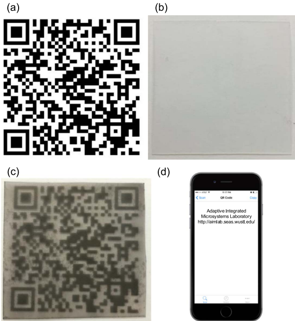
Fig. 5. Experiment showing different stages of QR self-assembly. (a) An example of QR code printed on a white paper (information encoded in this QR code: Adaptive Integrated Microsystems Laboratory http://aimlab.seas.wustl.edu/ ). (b) The same QR code printed on a plastic substrate using AuNR ink. (c) The plastic substrate after 20 min of silver-enhancement. (d) Information in the QR code decoded with a smart-phone app.
