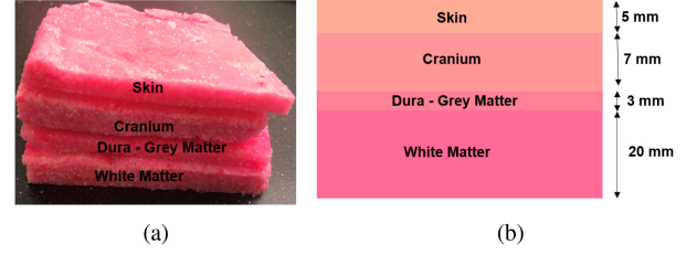
Fig. 13. (a) Head phantom tissue combination (b) dimensions of tissue combination used for the measurement.
