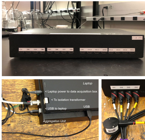
FIGURE 6. (Top) Front view of the as-built aggregation unit, with sixteen different HDMI channels enabling separate drive of each reader head. (Bottom left) External connections of the aggregation unit to the power line and the processing computer. (Bottom right) A prototype single-wavelength reader head (without the filter flipper) connected to the aggregation unit.
