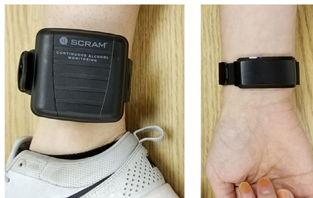
Fig. 1. AMS SCRAM ankle bracelet (left) and BACtrack Skyn wrist monitor (right) displayed side by side. The approximate weight of the devices is 6 oz (SCRAM) and 1 oz (Skyn prototype), respectively.
