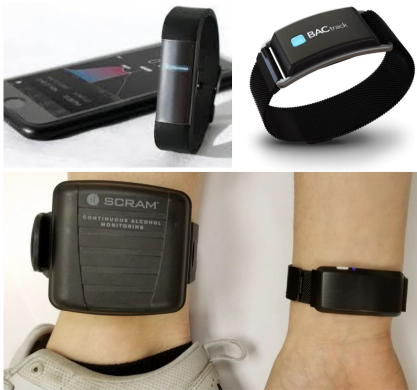
Figure 1 Top panel displays two new generation transdermal wrist sensors—Milo (left) and BACtrack (right). Bottom panel displays old-generation (AMS SCRAM; left) and new-generation (BACtrack Skyn prototype; right) devices to scale, side by side. Bottom panel adapted from [9] [Colour figure can be viewed at wileyonlinelibrary.com ]
