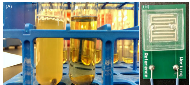
Figure 1 A, Dental implants immersed in bacteria (left, Implant #1) and control media (right, Implant #2). B, Biosensor used for metal ion detection. The sensor was fabricated at the University of Texas at Dallas in the Biomedical Micro-Devices and Nano-Technology Laboratory.
