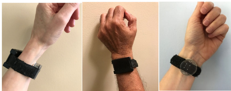
FIGURE 1 Pictures of alcohol biosensor monitor device WrisTAS™ showing black electronic box with battery and data storage and sensor (round clear disc).
