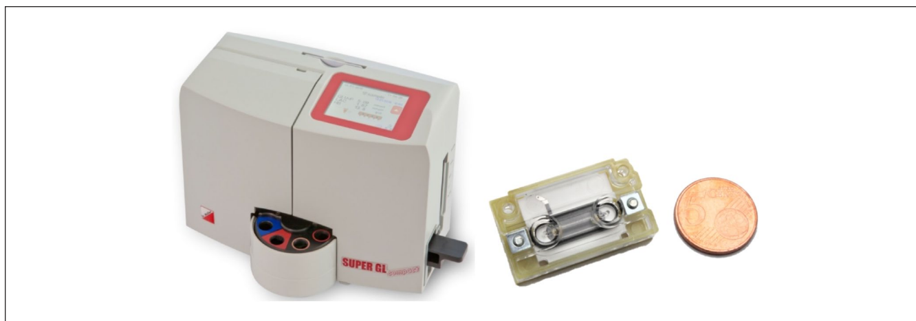
Figure 1. Pictures of the SUPER GL compact device and the biosensor (not to scale). Size of the device and biosensor: see Table 1.
