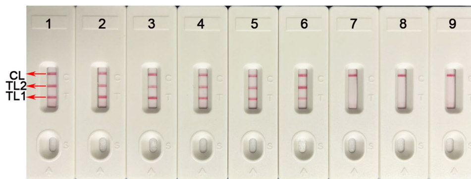
Fig. 4 Analytical sensitivity of mMCUDA assay using an AuNPs-LFA biosensor. The mMCUDA assay was performed using serial diluents of synthesized plasmids as templates ( 5 \times 10^5 to 5 \times 10^{-2} fg/ \mu\text{L} ). Biosensors 1–8 (A–C) correspond to 5 \times 10^5 , 5 \times 10^4 , 5 \times 10^3 , 5 \times 10^2 , 5 \times 10^1 , 5 \times 10^0 , 5 \times 10^{-1} , and 5 \times 10^{-2} fg/ \mu\text{L} . Strips 9 correspond to blank control (DNase/RNase-free water). As a result, the detection limit of the mMCUDA assay was 7.5 fg/reaction. mMCUDA, multiplex MCDA Combined with dUTP-aided UDGase and Detector-based AuNPs-LFA biosensor; MCDA, multiple cross-displacement amplification; AuNPs-LFA, gold nanoparticles-based lateral flow assay; TL1, test line 1; TL2, test line 2; CL, control line
