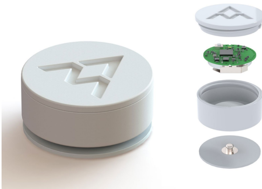
Fig. 1 Appearance of the PnuemoWave biosensor. The sensor can be seen on the left. On the right is the inside view of the biosensor, showing from top to bottom the housing lid, the accelerometer sensor, the sensor housing, and the ECG electrode used to mount the sensor onto the chest
