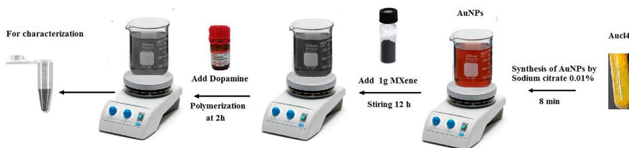
Fig. 1 Synthesis procedures of Ti3C2/AuNPs/PDA nanocomposite. The process begins with the reduction of tetrachloroauric acid (HAuCl 4 ) using trisodium citrate (Na 3 C 6 H 5 O 7 ) to produce AuNPs
