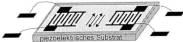
Fig. 10. Surface acoustic wave device (SAW). The acoustic shear wave and two interdigitated electrodes for the in- and outcoupling of the acoustic wave are depicted.
