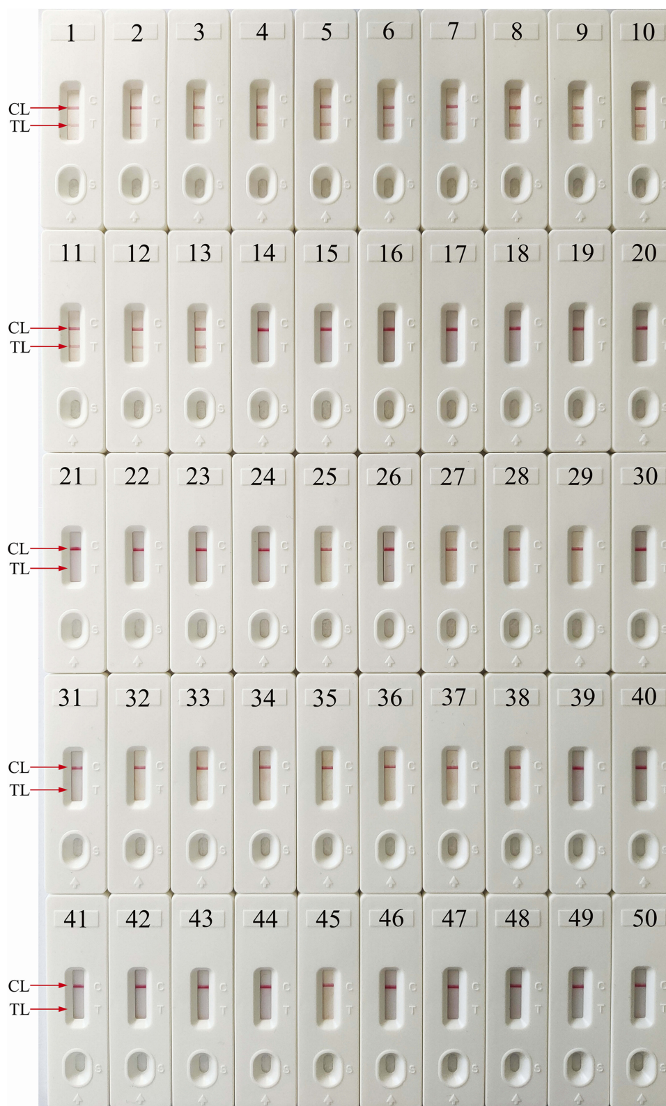
Figure 6 Specificity analysis of the E. faecalis -MCDA-LFB detection for different strains. The MCDA amplifications were carried out using different strain genomic DNA as templates and determined by means of visual LFB method. Biosensor 1, E. faecalis strain (ATCC 29212); biosensor 2–13, twelve isolated strain of E. faecalis from the Second Affiliated Hospital, Guizhou University of Traditional Chinese Medicine; biosensor 14–22, nine isolated Enterococcus faecium strains, biosensor 23–49, Enterococcus avium , Enterococcus raffinosus , Staphylococcus aureus , Pseudomonas aeruginosa , Legionella bacillus , Hemophilus parainfluenza , Bordetella parapertussis , Klebsiella pneumonia , Shigella boydii , Mycoplasma pneumonia , Enteropathogenic Escherichia coli , Streptococcus pneumonia , Staphylococcus saprophyticus , Enterotoxigenic Escherichia coli , Invasive Escherichia coli , Enterohemorrhagic Escherichia coli , Enterococcal Escherichia coli , Streptococcus suis , Vibrio cholera , Acinetobacter baumannii , Bacillus cereus , Vibrio parahaemolyticus , Shigella flexneri , Listeria monocytogenes , Mycobacterium tuberculosis , Leptospira interrogans , Brucella suis ; biosensor 50, blank control (DW).
