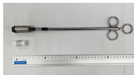
Figure 1. The biosensor is equipped with a triaxial accelerometer and a temperature sensor, along with its injector for oral administration in calves. A ruler is included for scale.
