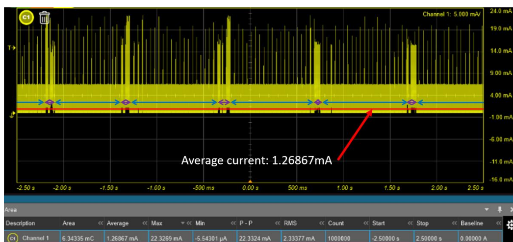
Figure 16. Current consumption of the surface EMG system. The blue line is only ADC conversion and the purple line is BLE transmission and ADC conversion.
