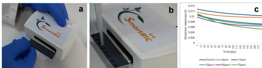
Figure 1. (a) The portable potentiometric biosensor device with the disposable sensor strip. (b) Membrane-engineered cells and sample were placed on the top of each of the eight carbon screen-printed electrodes for simultaneous measurements. (c) Testing results are displayed in real time on screen, as a voltage vs. time graph, and stored for later processing.
