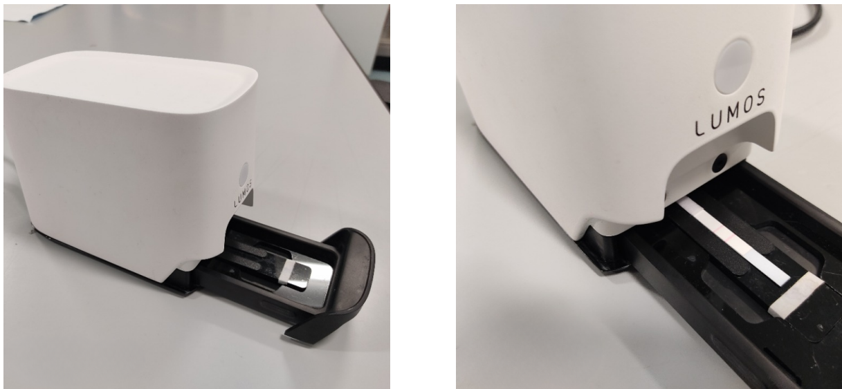
Figure 2. Lumos Reader device for capturing LFA images.
