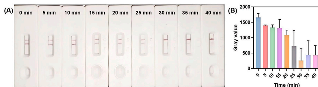
Figure 6. Optimization of reaction time for RPA-CRISPR/Cas12a system. (A) Visual detection results for various cleavage durations. (B) Quantitative gray value measurements of the T zone signal over different reaction times.
