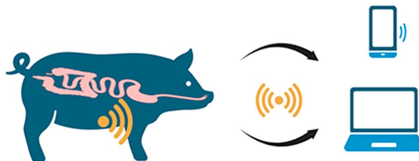
Figure 9. Ingestible micro-bio-electronic device (IMBED) for heme in vivo monitoring. The swine intestine was colonized with a transformed probiotic E. coli strain that senses heme due to the heterologous expression of the Lactococcus lactis heme-responsive transcriptional repressor (HrtR protein). After the microelectronics-equipped capsule deposition the heme level was transmitted to a laptop or a cellular phone. Illustration adapted from [106] and created in BioRender. Vidic, J. (2025) https://BioRender.com/2zu2dh5 .
