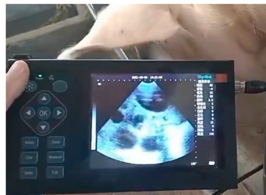
Figure 3. Data acquisition, artifacts, and AI enhancement results. (A) The ultrasound phantom model used for supplemental data collection, A raw B-mode image from the phantom. (B) photograph of acquisition of B-ultrasound image of a pregnant sow using an ultrasonic sector scanning probe, A raw B-mode image from a sow, showing a gestational sac (yellow circle) obscured by reverberation artifact.
