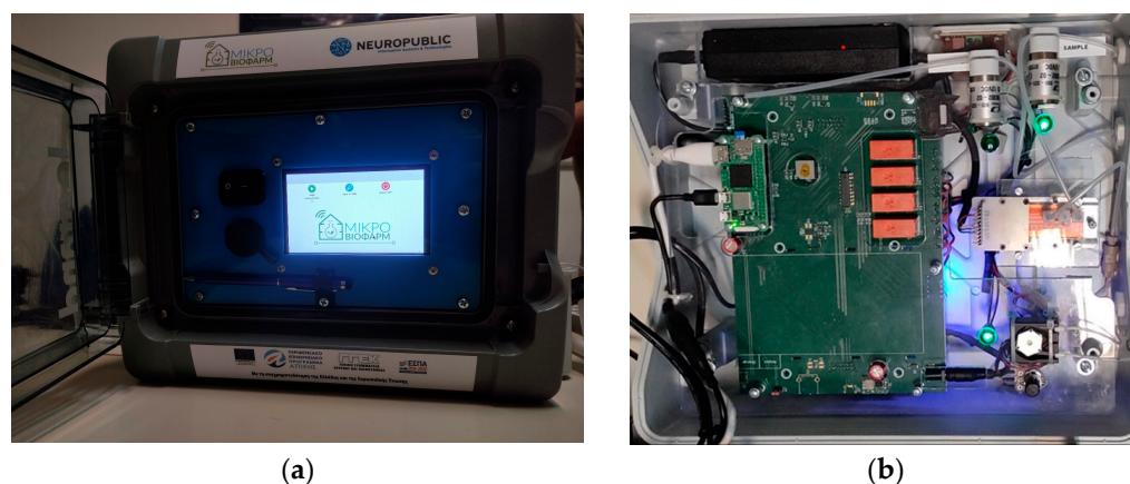
Figure A1. Overview of the standalone LoC system. (a) The complete system housed in a waterproof electrical enclosure as well as the LCD display interface for real-time monitoring; and (b) the integrated system components.
