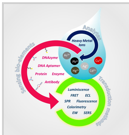
Figure 1. Optical biosensor scheme strategies for heavy metal (HM) ion detection in a water/milk “drop”. Transduction methods and bioreceptor classes synergistically employed for the development of recently published devices.
