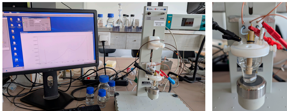
Figure 3. Photos of the measuring system and electrochemical cell with a set of three electrodes.
