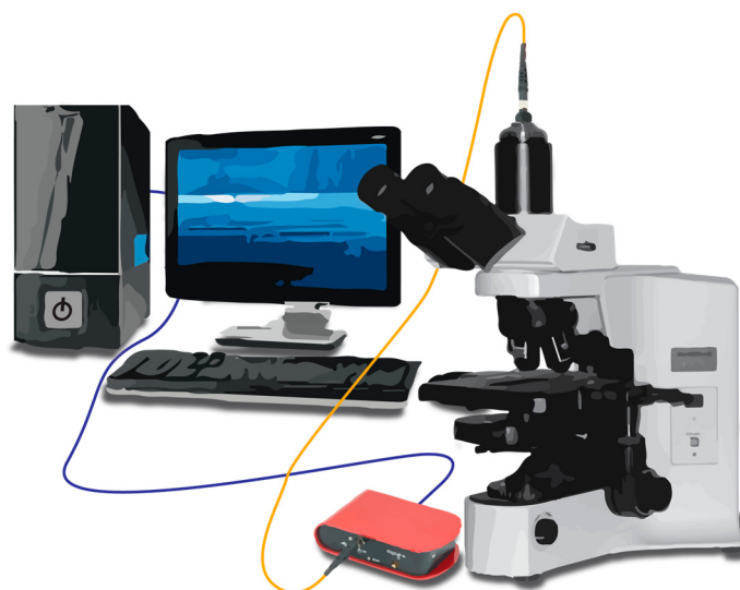
Figure 4. Visual representation of the optical setup for plasmonic sensor measurements, featuring a broad-spectrum visible light source, a microscope, a spectrometer, and an optical fiber.
