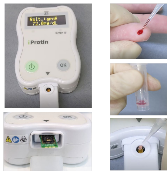
Figure 2. Operation of the iProtein reader with ApoB SH-SAW biosensor.
