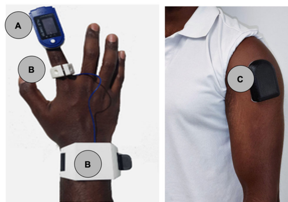
Figure 1. (A) Commercial pulse oximeter control; (B) Prototype-ring configuration; (C) Prototype-shoulder configuration.
