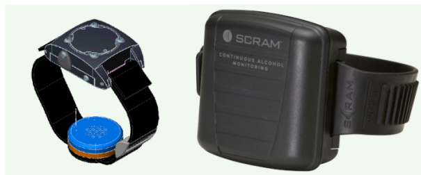
FIGURE 1. Left: Giner inc. WrisTAS 7 transdermal alcohol monitoring biosensor. Right: Alcohol Monitoring Systems Secure Continuous Remote Alcohol Monitor (SCRAM) transdermal alcohol biosensor system.
